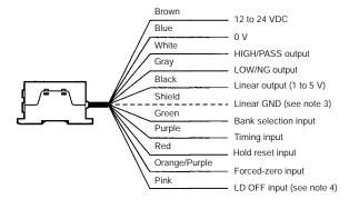
**Note: 1.** When particularly high resolutions are required, use a separate, stable power supply.
