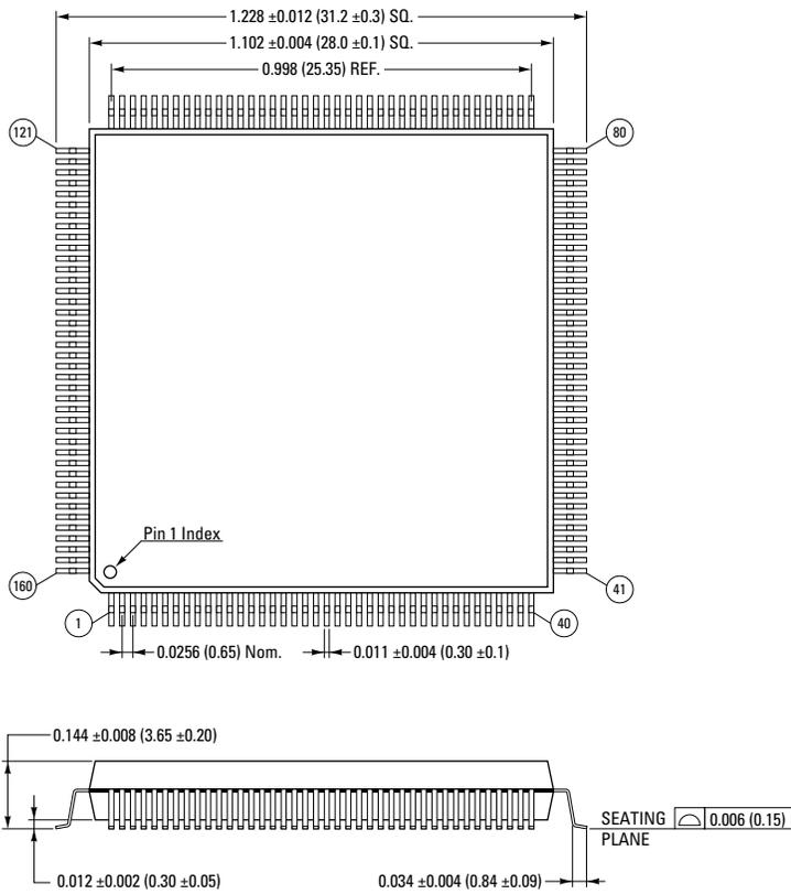
Dimensions in inches, dimensions in brackets in (millimeters).
