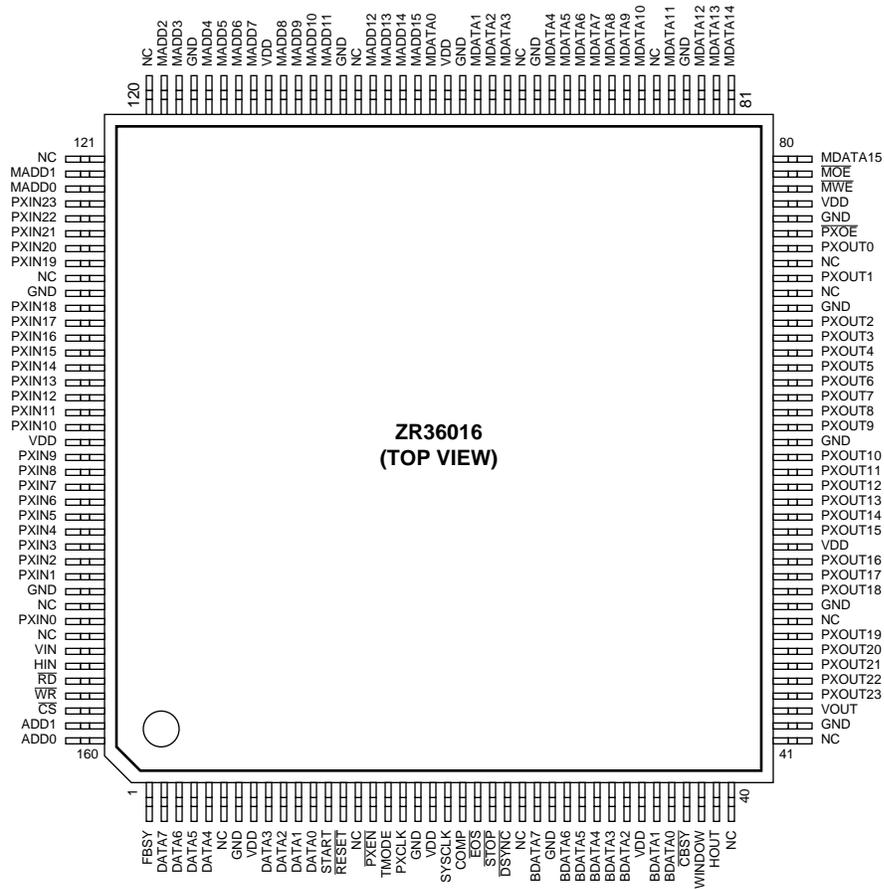
Figure 41. ZR36016 Plastic Quad Flat Pack Pinout
