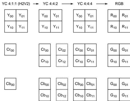
The components in dashed boxes are used when SBFL=1, to compute Cr<sub>01</sub>, Cr<sub>11</sub>, Cb<sub>01</sub> and Cb<sub>11</sub>.
