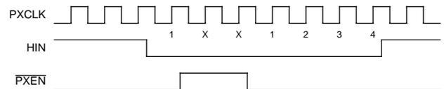
**Figure 11. Effective PXCLK Cycles (4 Effective Cycles)**
