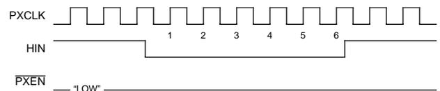
**Figure 10. Effective PXCLK Cycles (6 Effective Cycles)**
