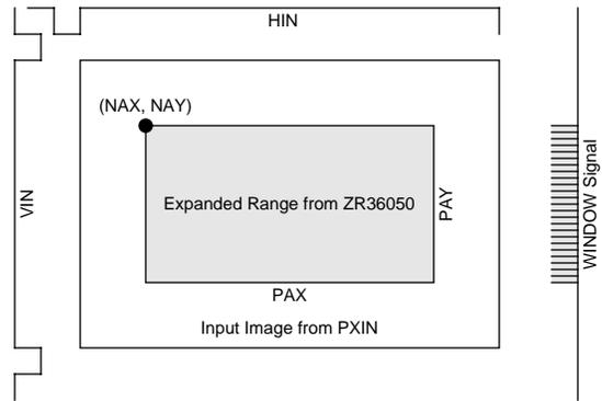
**Figure 16. Overlay of Expanded Image on PXIN**
