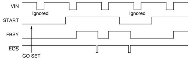
Figure 21. Sequential Mode Operation (CNTI = 1) with START Control
