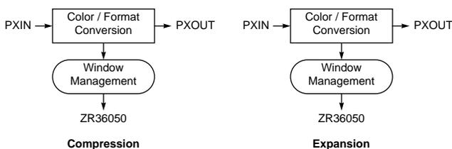
**Figure 15. Data Flows Between PXIN, PXOUT and ZR36050**
