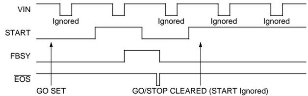
Figure 22. Sequential Mode Operation with GO/STOP Control
