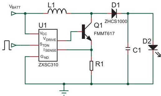
This circuit provides a continuous current output to the LED by rectifying and buffering the DC-DC output. This ensures maximum LED brightness.
