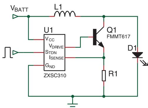
To ensure optimum efficiency, and therefore maximum battery life, the LED is supplied with a pulsed current. Maximum efficiency is ensured with the removal of rectifier losses experienced in the maximum brightness solution.
