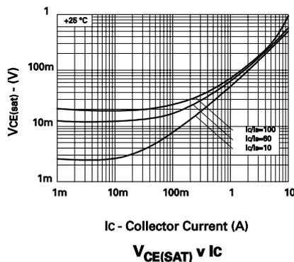
The Zetex FMMT617 is an ideal choice of transistor, having a low saturation voltage. A data sheet for the FMMT617 is available on Zetex web site or through your local Zetex sales office. Outline information is included in the characteristics section of this data sheet.
