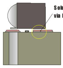
Solder paste are on via hole area.
