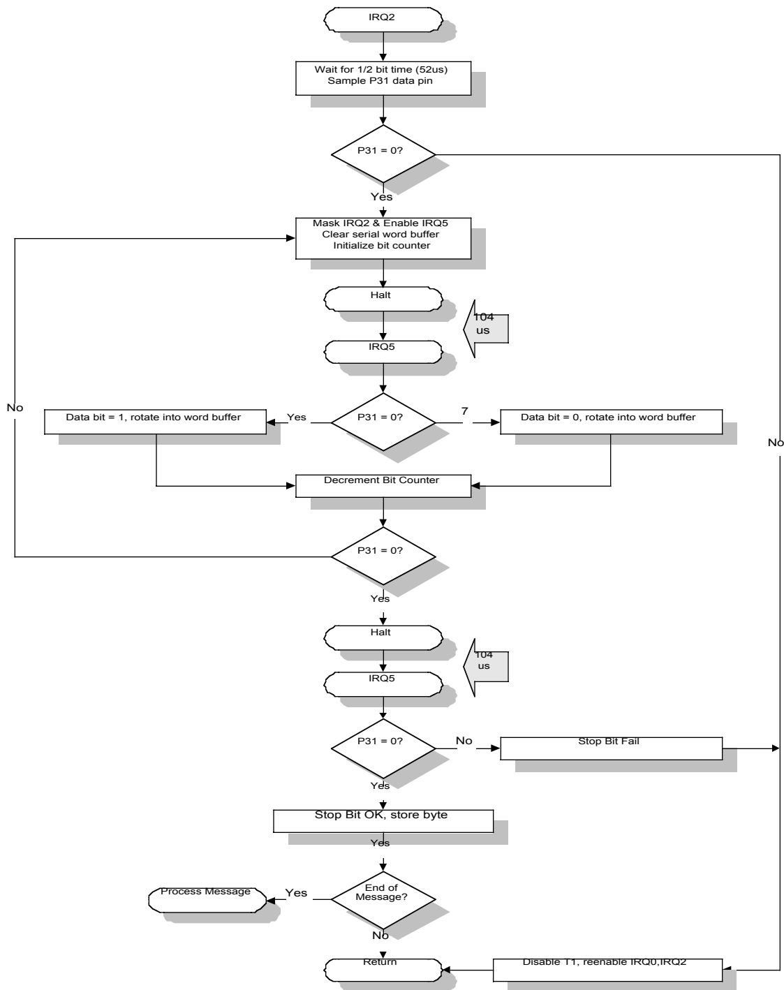
Figure 3. Receiving RF Serial Communication Flow Diagram
