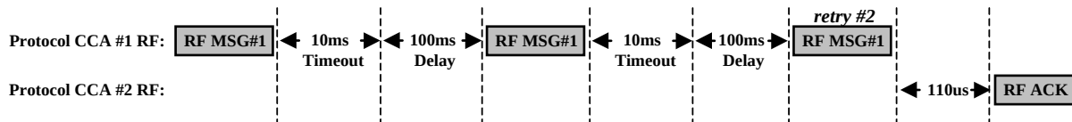
Figure 7. RF Retry Timing
