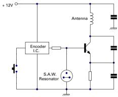
The majority of modem automotive alarms employ coded RF systems that key a VHF carrier wave with a unique (or at least, one of many) code. The encoding ICs available are able to keep component count to a minimum, and for efficient, cost-effective and non-critical operation, a high performance RF driver is therefore essential.
