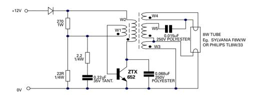
Fluorescent tubes are notoriously difficult loads to drive. Before striking, the tube effectively appears open circuit, needing 300V or greater to provoke conduction. After striking they adopt a low voltage characteristic where the required current can be sustained at low voltage, typically 40V. These changes in characteristics place severe demands on any DC-AC converter and the associated transistors used to drive the tubes.
