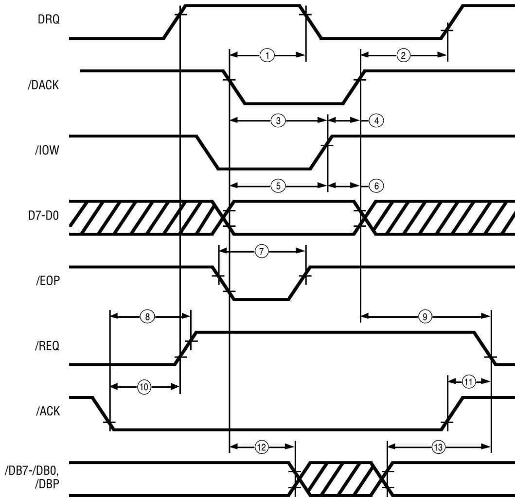
Figure 46. DMA Write (Non-Block Mode) Target Send Cycle
