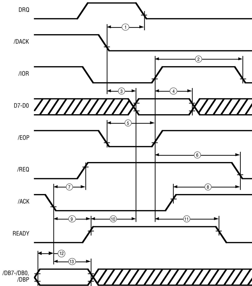
Figure 51. DMA Read (Block Mode) Target Receive Cycle
