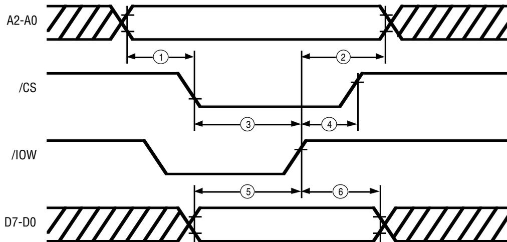
Figure 44. CPU Write Cycle
