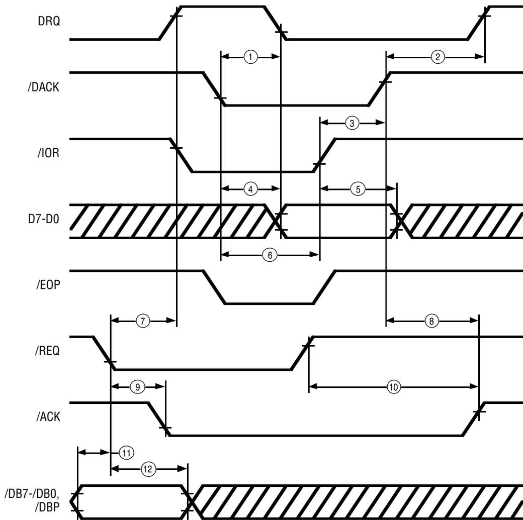
Figure 49. DMA Read (Non-Block Mode) Initiator Receive Cycle
