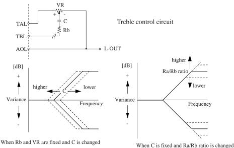
Ra is the resistor shown in the "Bass control circuit diagram"
