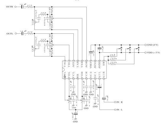
YSS906 can be made different characteristics with external components at various values.
