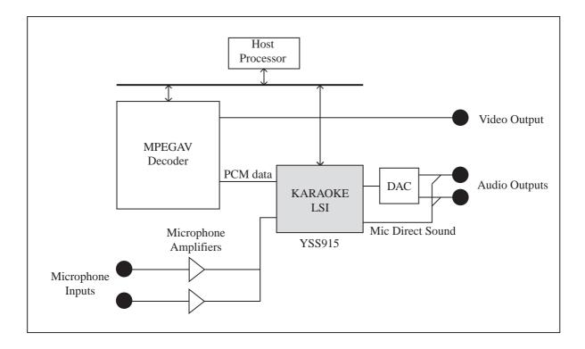
For this LSI, audio signal is inputted as digital signal, and vocal signal from the microphone is inputted as analog signal.
