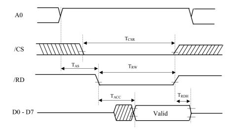
Note:  $T_{ACC}$  is defined with respect to the moment /CS or /RD becomes Low level later.  $T_{CSR}$ ,  $T_{RW}$  and  $T_{RDH}$  are defined with respect to the moment /CS or /RD becomes High level.
