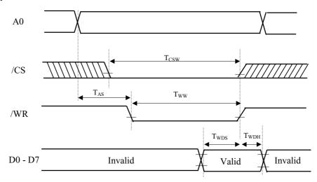
Note:  $T_{CSW}$ ,  $T_{WW}$ , and  $T_{WDH}$  are defined with respect to the moment /CS or /WR becomes High level.
