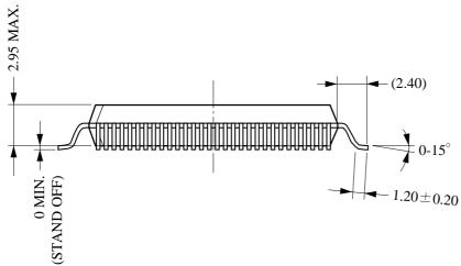
The figure in the parenthesis ( ) should be used as a reference. Plastic body dimensions do not include burr of resin. UNIT: mm
