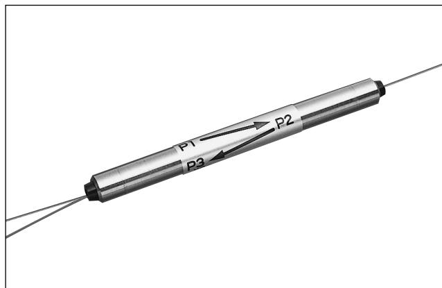
This optical circulator is a passive device for optical transmission systems, applying the Faraday effect of LPE film. It has attained outstanding characteristics (high isolation, low insertion loss) and compact size.
