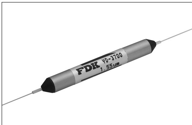
The YD-3700 is a polarization-independent optical isolator for optical communications. Using FDK's original precision fiber collimator in its input / output section, the YD-3700 has attained a high isolation and a low insertion loss. Further, its laser-welded inner connection ensures a superb reliability and durability. Besides the product uses LPE films.
