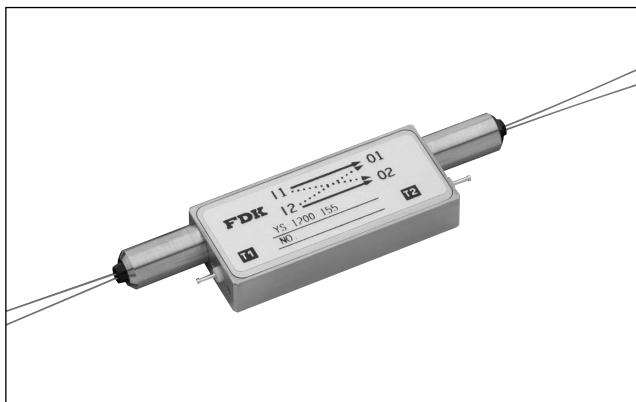
These optical switches are self latching type applying the Faraday effect of LPE film. Due to the exclusion of any moving parts based non-mechanical structures, they have attained a high reliability and rapid switching speed, and furthermore, using the two-hole ferrule collimator, attained high isolation, low insertion loss and compact size.
