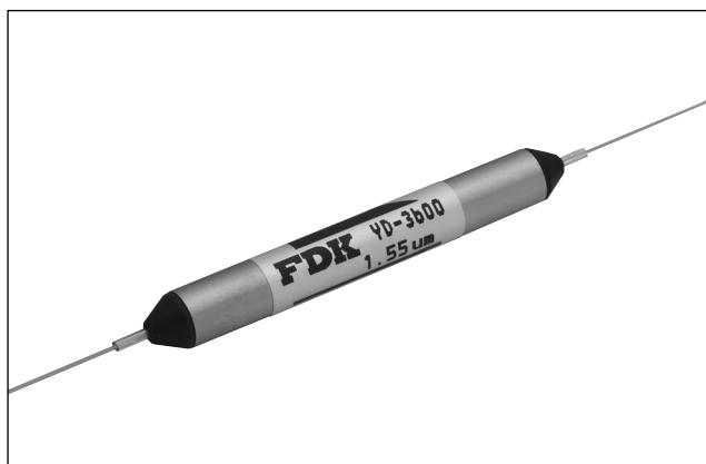
The YD-3600 is a polarization-independent optical isolator for optical communications. Using FDK's original precision fiber collimator in its input / output section, the YD-3600 has attained a high isolation and a low insertion loss. Further, its laser-welded inner connection ensures a superb reliability and durability. Besides the product uses LPE films.
