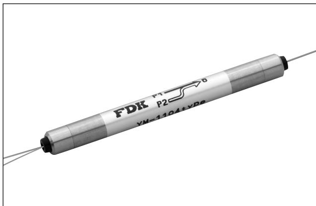
The YM-1101 and YM-1104 are polarization combiners. For an optical fiber amplifier, a high optical pump power is needed to obtain high gain. Polarization combiners combine two polarized pump sources into one and they yield single high pump power.
