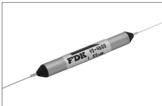
The YD-4600 is a polarization-independent optical isolator used in optical communications. Using FDK's original precision fiber collimator in its input / output section, the YD-4600 has attained a high isolation and a low insertion loss. Further, its laser-welded inner connection ensures a superb reliability and durability. Besides the product uses LPE films.
