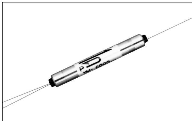
Optical signal amplification in optical transmission lines is carried out by optical fiber amplifiers (EDFA). The YM-6000 type, which is the combination of an isolator and a WDM filter, is connected to the amplifier to assist it by backward pumping.
