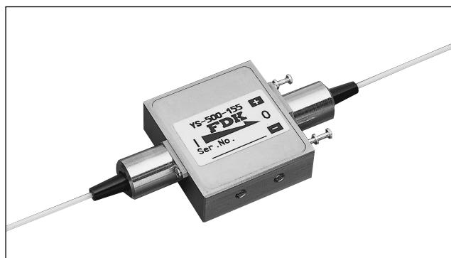
The YS-500 is a variable optical attenuator applying the Faraday effect of LPE film. The attenuation levels can be adjusted continuously by current control. Due to the exclusion of any moving parts, it has attained a high reliability and rapid response time.
