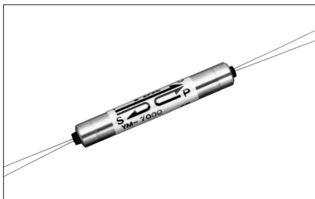
Optical signal amplification in optical transmission lines is carried out by optical fiber amplifiers (EDFA). The YM-7000 type, which is the combination of an isolator, a coupler and a WDM filter, is connected to amplifier to assist its performance by forward pumping.
