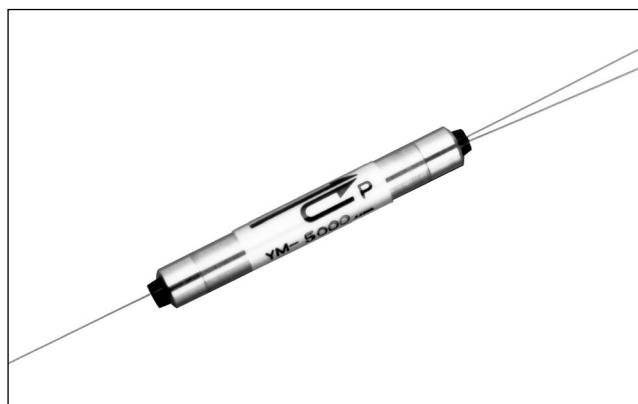
Optical signal amplification in optical transmission lines is carried out by optical fiber amplifiers (EDFA). The YM-5000 type, which is the combination of an isolator and a WDM filter, is connected to the amplifier to assist it by forward pumping.
