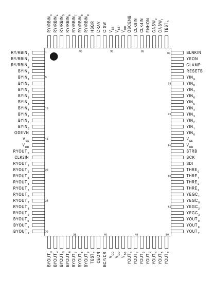
Package: 100-pin PQFP.  $\theta_{ja} = xx \circ C/watt$
