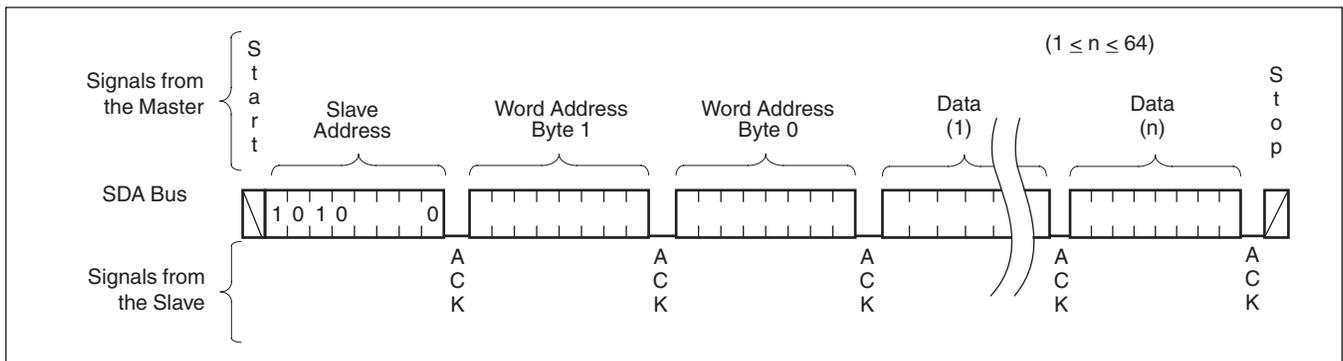
Figure 10. Writing 12 bytes to a 64-byte page starting at location 60.
