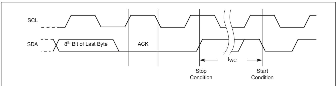
Nonvolatile Write Cycle Timing
