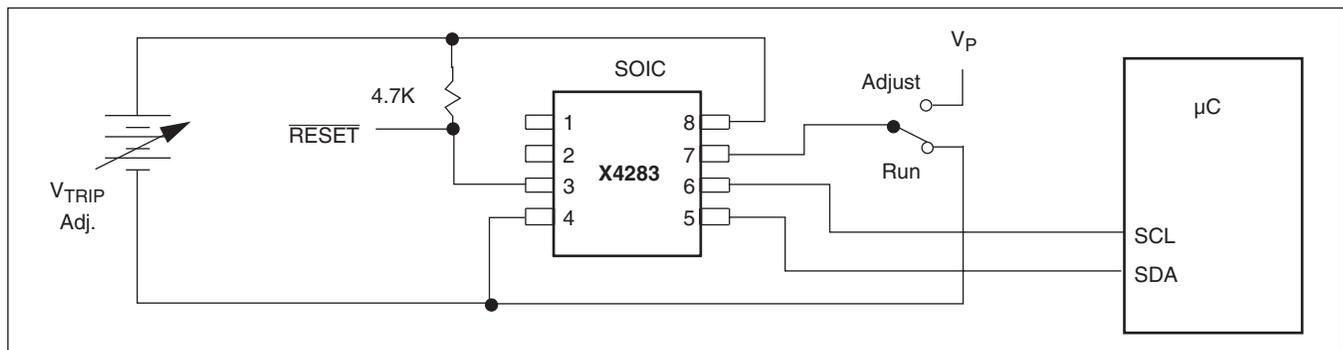
Figure 4.  $V_{TRIP}$  Programming Sequence
