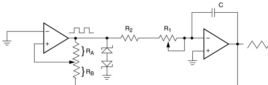
$$\text{frequency} \propto R_1, R_2, C$$
