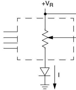
Two terminal Variable Resistor;
