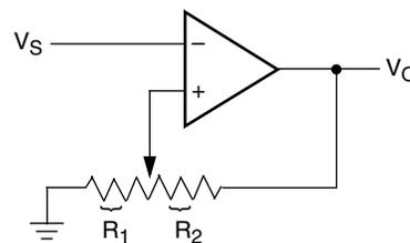
$$V_{UL} = \{R_1 / (R_1 + R_2)\} V_O (\text{max})$$
