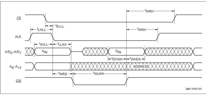
**Note:** (7) two is the minimum cycle time to be allowed from the system perspective unless polling techniques are used. It is the maximum time the device requires to automatically complete the internal write operation.
