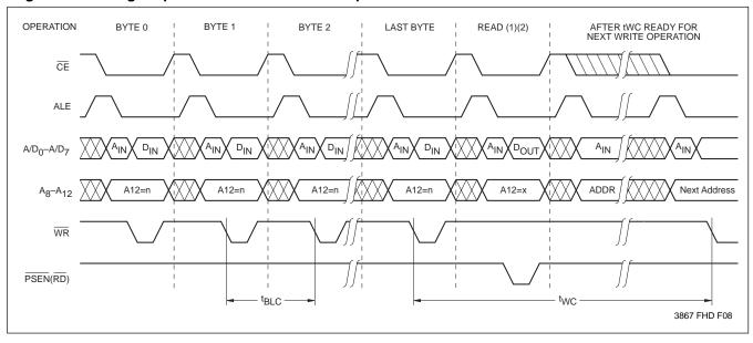
**Notes:** (1) For each successive write within a page write cycle A<sub>5</sub>–A<sub>12</sub> must be the same.
