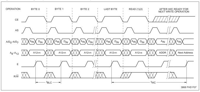
**Notes:** (1) For each successive write within a page write cycle A<sub>5</sub>–A<sub>12</sub> must be the same.
