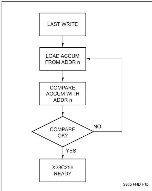
The Toggle Bit can eliminate the software housekeeping chore of saving and fetching the last address and data written to a device in order to implement  $\overline{DATA}$  Polling. This can be especially helpful in an array comprised of multiple X28C256 memories that is frequently updated. The timing diagram in Figure 4 illustrates the sequence of events on the bus. The software flow diagram in Figure 5 illustrates a method for polling the Toggle Bit.
