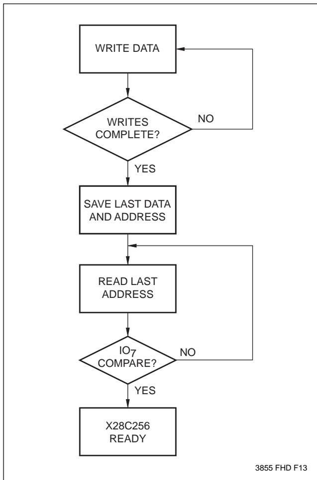
DATA Polling can effectively halve the time for writing to the X28C256. The timing diagram in Figure 2 illustrates the sequence of events on the bus. The software flow diagram in Figure 3 illustrates one method of implementing the routine.
