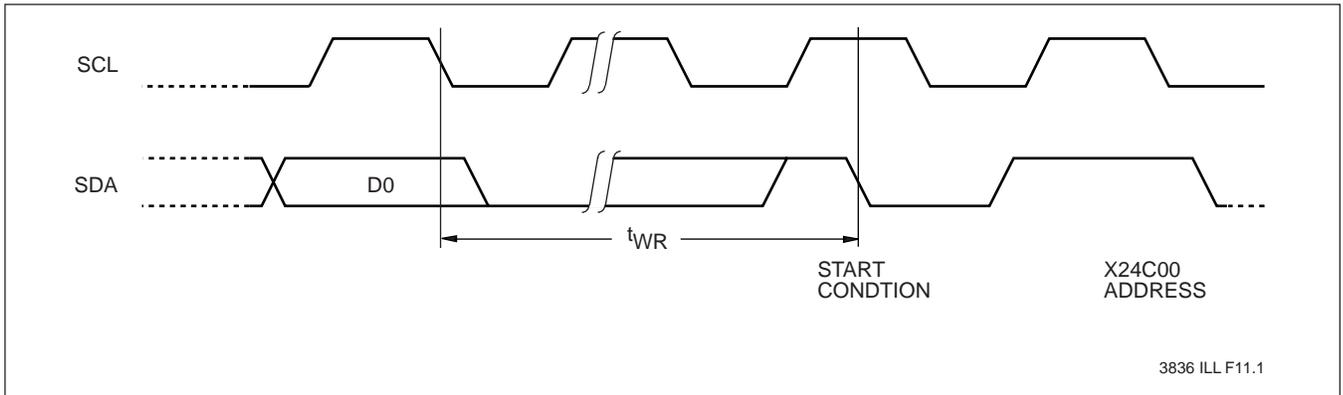
**Note:** (4) The write cycle time is the time from the initiation of a write sequence to the end of the internal erase/program cycle. During the write cycle, the X24C00 bus interface circuits are disabled, SDA is high impedance, and the device does not respond to start conditions.
