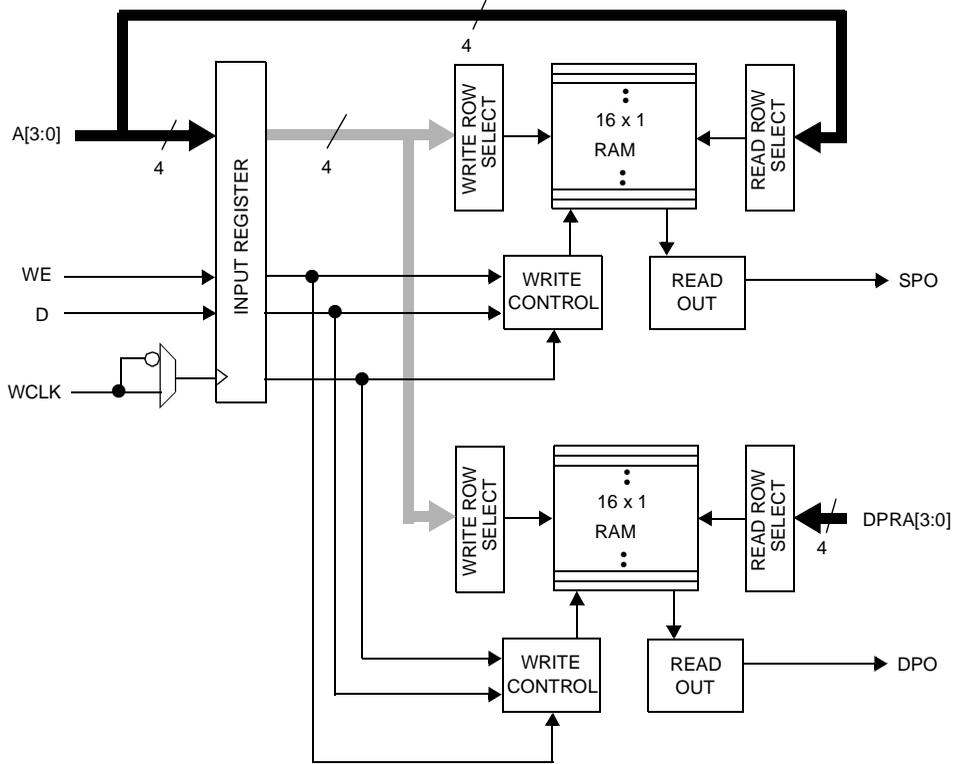
**Figure 14: Logic Diagram for the Dual-Port RAM**
