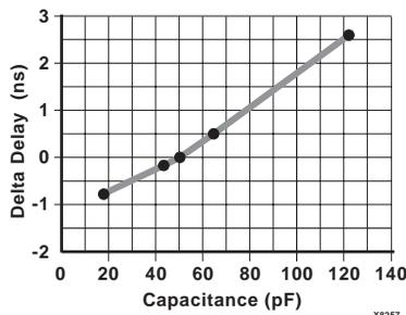
**Figure 33: Delay Factor at Various Capacitive Loads**
