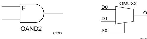
**Figure 7: AND & MUX Symbols in Spartan-XL IOB**
