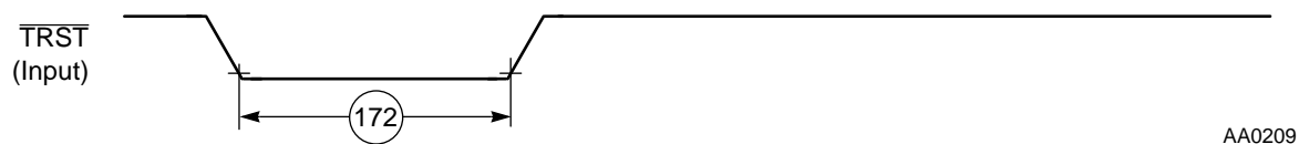
Figure 2-33 \overline{\text{TRST}} Timing Diagram
