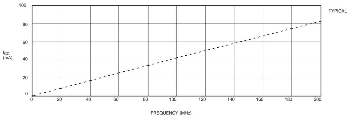
Figure 5:  $I_{CC}$  vs. Frequency at  $V_{CC} = 5V$ ,  $25^{\circ}C$
