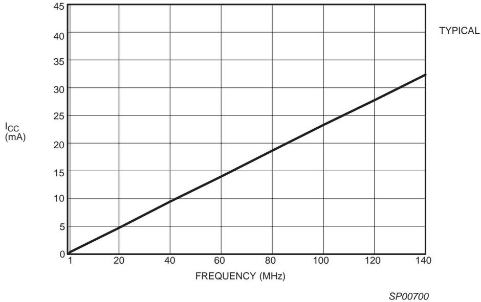
**Figure 5: I<sub>CC</sub> vs. Frequency at V<sub>CC</sub> = 3.3V, 25°C**
