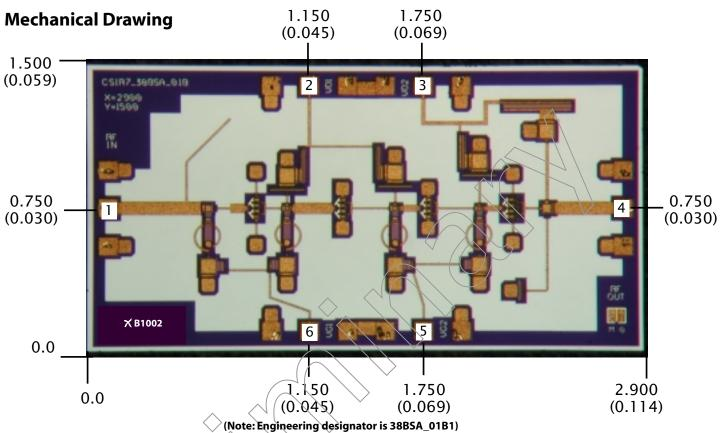
Units: millimeters (inches) Bond pad dimensions are shown to center of bond pad. Thickness: 0.100 (0.004) (for reference only), Backside is ground, Bond Pad/Backside Metallization: Gold All Bond Pads are 0.100 x 0.100 (0.004 x 0.004).
