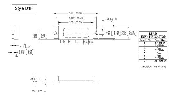
This model is available in the D1F (H11822) and D2F (H12048) package styles. Style D1F is shown here for reference only. Style D2F is the same except the three ground leads are not present.
