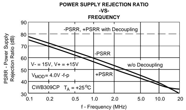
By inserting 1K ohm resistors in series with V+ and V- power supply lines and decoupling both pins at the device socket, it is possible to improve power supply rejection ratios of a video switch by 50dB at frequencies of 20MHz and higher.
