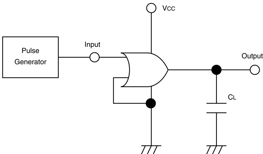
Note: open output when measuring supply current
