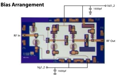
**Bypass Capacitors** – Recommended Capacitors can be found at Presidio Components (www.presidiocomponents.com)
