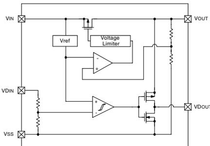
(2) XC66DN N-ch open drain
