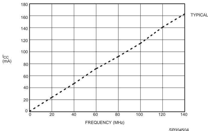
Figure 5: V<sub>CC</sub> vs. Frequency at V<sub>CC</sub> = 5.0V, 25°C
