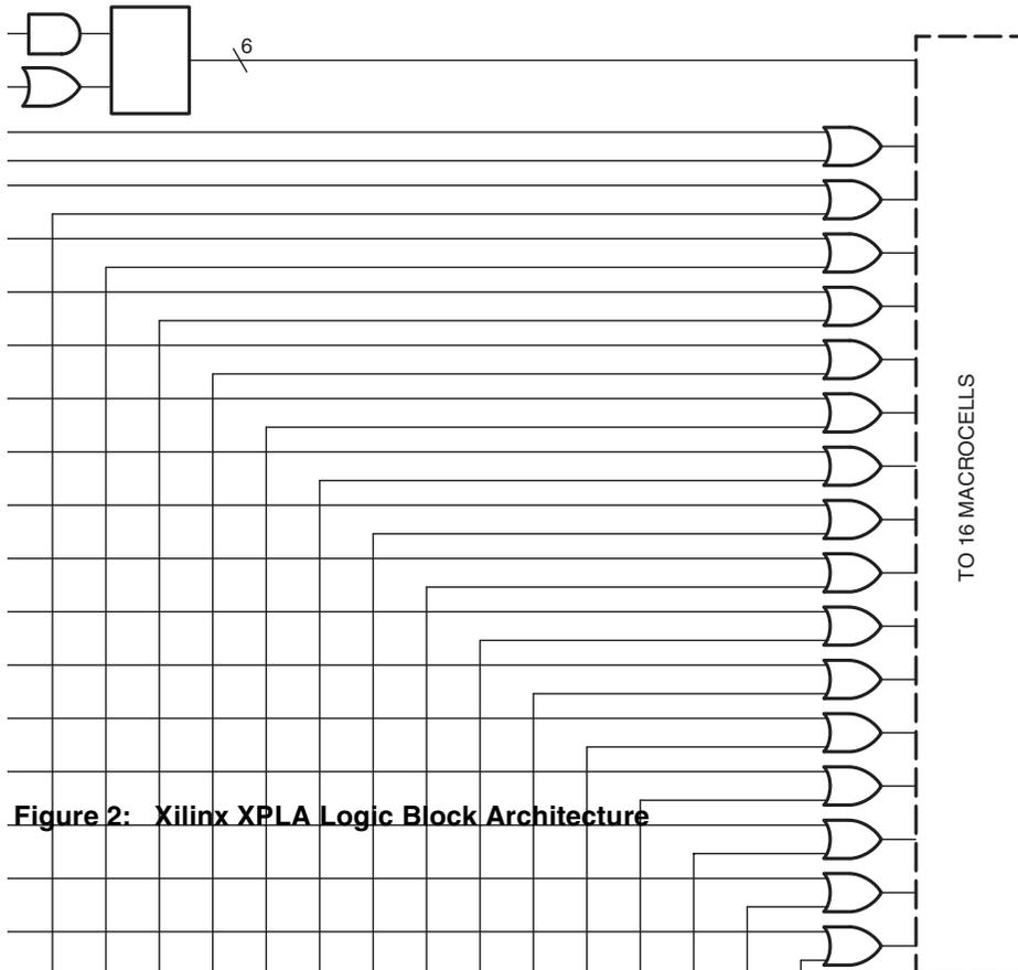
Figure 2: Xilinx XPLA Logic Block Architecture
