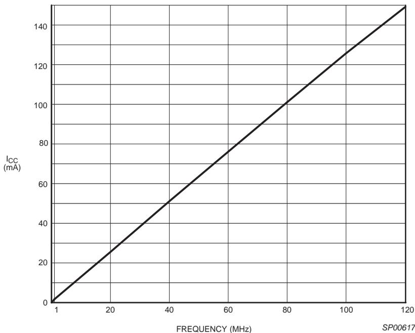
**Figure 5:**  $I_{CC}$  vs. Frequency at  $V_{CC} = 5.0V$ , 25°C
