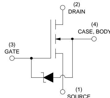
BODY INTERNALLY CONNECTED TO CASE.
