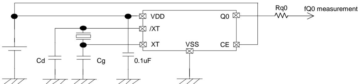
\* Please use oscillation capacitors  $C_g$ ,  $C_d = 10\text{pF}$  externally
