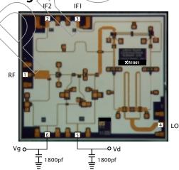
**Bypass Capacitors** – Recommended Capacitors can be found at Presidio Components (www.presidiocomponents.com)
