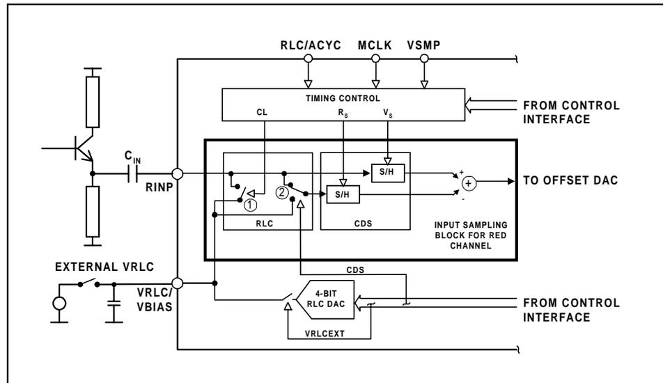
**Figure 7 Reset Level Clamping and CDS Circuitry**
