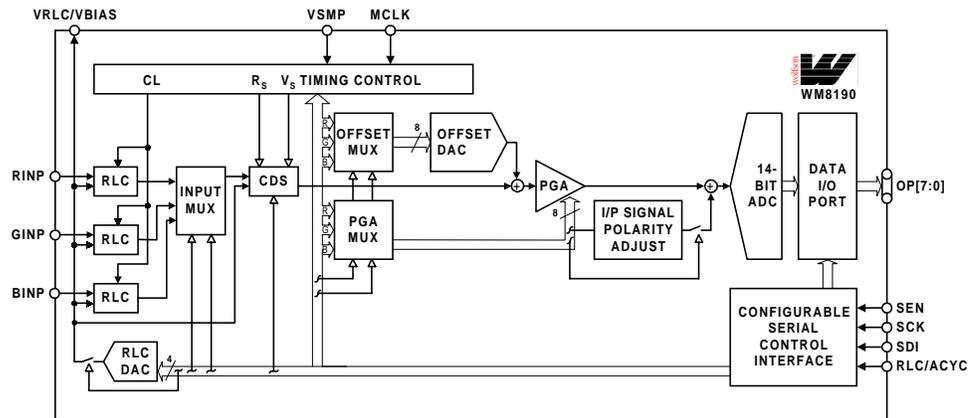
Figure 16 Signal Path When in Line-by-Line Mode
