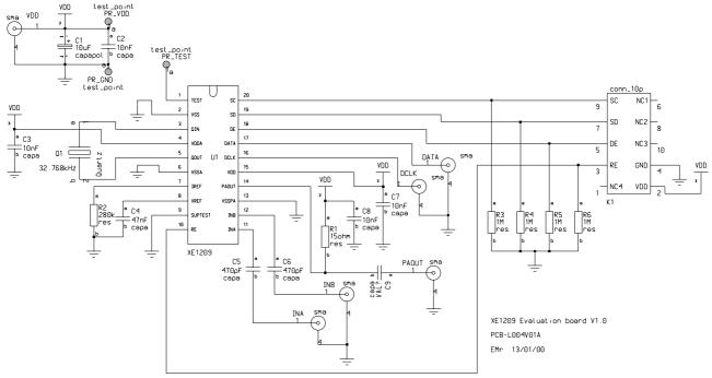
Note: pins TEST and SUPTEST remain unconnected
