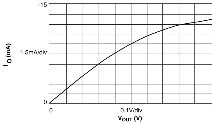
**Figure 10. Output Sink Current vs. Output Voltage**
