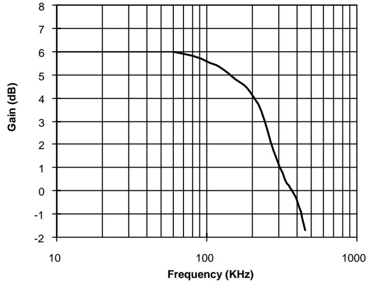
Figure 14. Closed Loop Gain vs. Frequency
