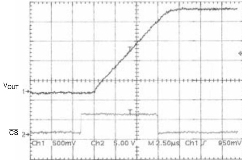
Figure 12. Voltage Output Settling Time ( $t_s$ ),
