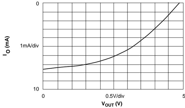
**Figure 9. Output Source Current vs. Output Voltage**
