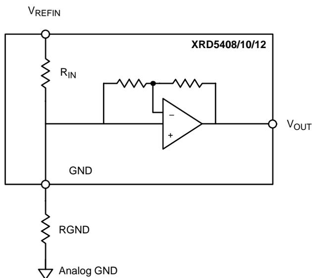
**Figure 6. AC<sub>FT</sub> Feedthrough Equivalent Circuit, DAC Code = 0**
