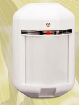
Get reliable detection and freedom from false alarms with Aleph's Unicorn XP-40 Series Pet Immune Detector loaded with unique innovations. Superior white-light and RFI immunity, SMD circuitry, and unique copper-plated circuit board provide outstanding performance and sensitivity. The low-cost XP-40 Series incorporates a fully tested dual pyroelectric element, jumper selectable 2/4 pulse count, and a walk-test LED.
