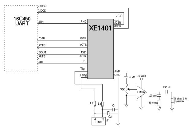
Note: RJ11 Pin assignments reflect a 6-pin connector. Tip and Ring are always the center pins of the RJ11 jack.
