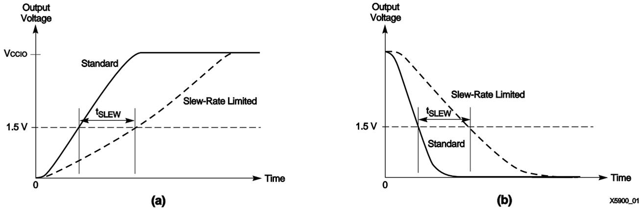
Figure 12: Output Slew-Rate Control For (a) Rising and (b) Falling Outputs
