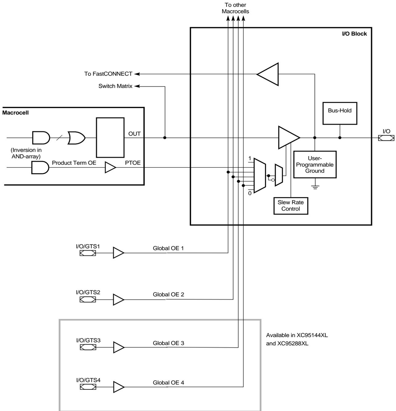
**Figure 10: I/O Block and Output Enable Capability**
