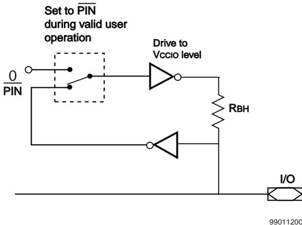
Figure 13: Bus-Hold Logic
