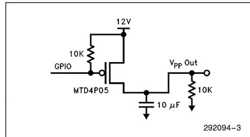
**Figure 3. V<sub>pp</sub> Switch Schematic**
