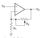
$V_{O} = (1 + R_{2}/R_{1})V_{S}$
