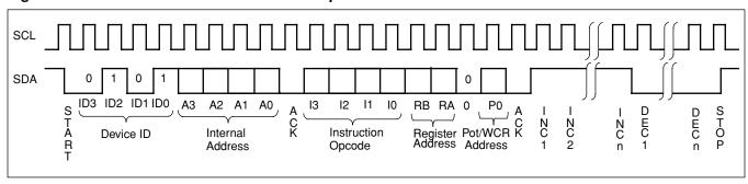
Figure 6. Increment/Decrement Timing Limits
