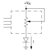
Two terminal Variable Resistor; Variable current
