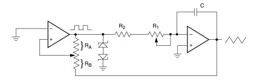
$\begin{array}{l} \text{frequency} \propto R_1,\,R_2,\,C \\ \text{amplitude} \propto R_A,\,R_B \end{array}$
