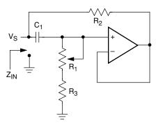
$$\begin{split} Z_{IN} = R_2 + s \; R_2 \; (R_1 + R_3) \; C_1 = R_2 + s \; Leq \\ (R_1 + R_3) >> R_2 \end{split}$$
