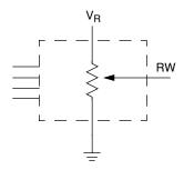
Three terminal Potentiometer; Variable voltage divider
