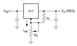
$V_{O}(REG) = 1.25V(1+R_{2}/R_{1})+I_{adj}R_{2}$
