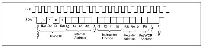
Figure 4. Three-Byte Instruction Sequence
