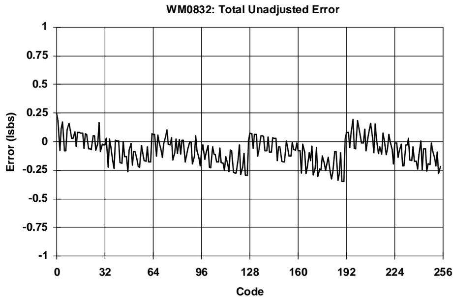
Test conditions:  $V_{CC} = 5V$ ,  $V_{REF} = 5V$ , Temp = 25°C,  $F_{CLK} = 250KHz$
