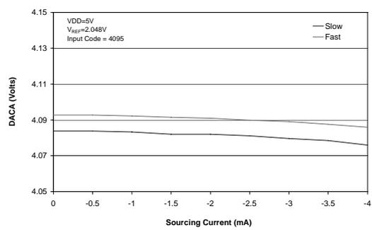
Figure 6 Output Load Regulation (Source) AVDD = 5V
