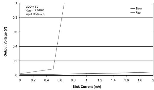
Figure 4 Output Load Regulation (Sink) AVDD = 5V
