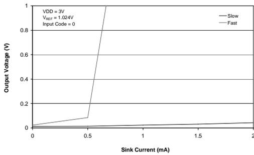
Figure 3 Output Load Regulation (Sink) AVDD = 3V
