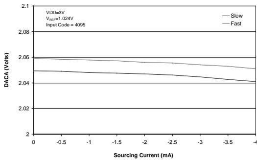
Figure 5 Output Load Regulation (Source) AVDD = 3V
