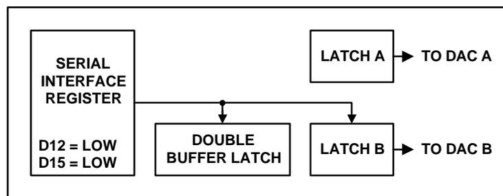
Figure 8 Latch B and Double Buffer Write
