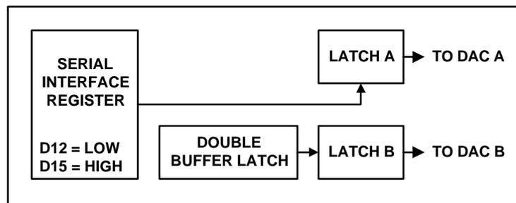
Figure 7 Latch A Write, Latch B Update
