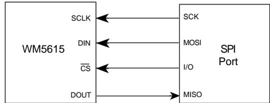
Figure 3 - SPI/QSPI Connection
