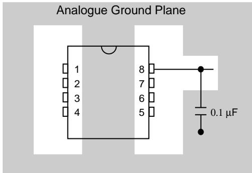
Figure 5 - Power-Supply Bypassing
