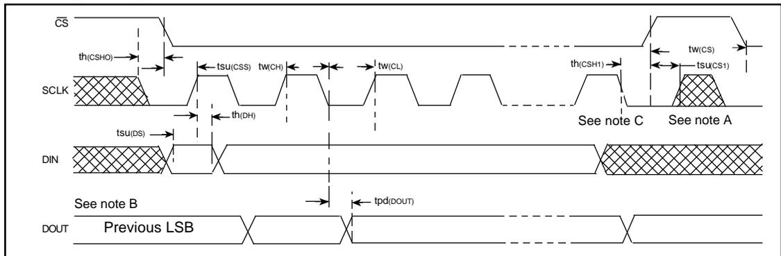
NOTES: A. The input clock, applied at the SCLK terminal, should be inhibited low when CS is high to minimise clock feedthrough.
