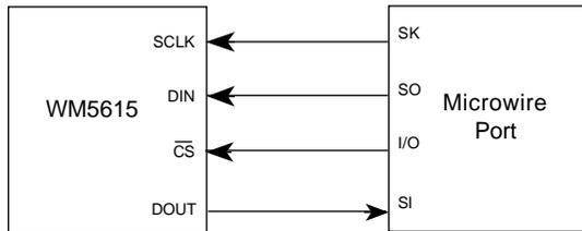
Figure 2 - Microwire Connection
