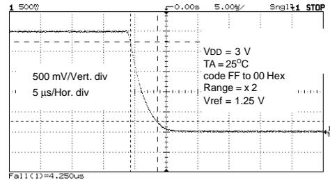
Fall time = 4.25  $\mu\text{s}$ , Negative slew rate = 0.46  $\mu\text{s}$
