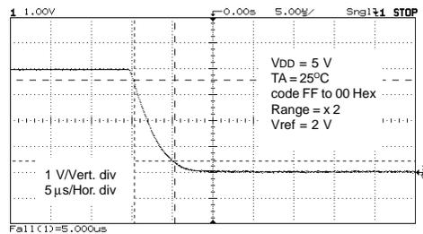
Fall time = 5.0  $\mu\text{s}$ , Negative slew rate = 0.63  $\mu\text{s}$
