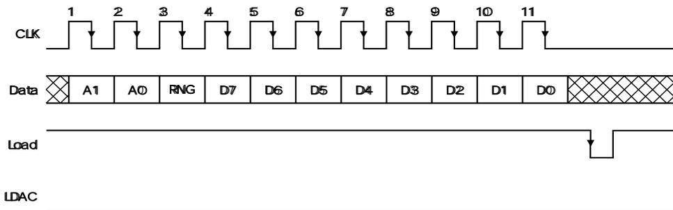
Figure 1. Load controlled update (LDAC = 0)
