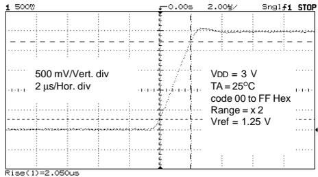
Rise time = 2.05  $\mu\text{s}$ , Positive slew rate = 0.96  $\mu\text{s}$
