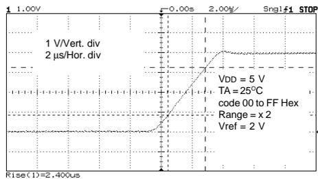
Rise time = 2.4  $\mu\text{s}$ , Positive slew rate = 1.0  $\mu\text{s}$
